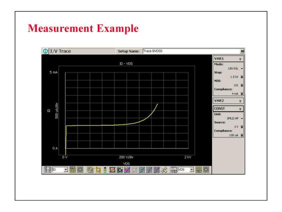
Perform measurement. The graph area will show the measurement result as shown in this example.
