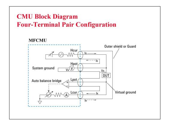
Generally, any mutual inductance, interference of the measurement signals, and unwanted residual factors in the connection method incidental to ordinary termination methods will have significant effects on the measurements, especially at a high frequency. The MFCMU employs the four-terminal pair (4TP) measurement configuration which permits easy, stable, and accurate measurements and avoids the measurement limitations inherent to such factors.
