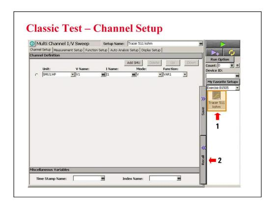
The Tracer Test setup can be recalled in the Tracer Test mode as shown in the previous page. Also it can be recalled and used in the Classic Test mode.
