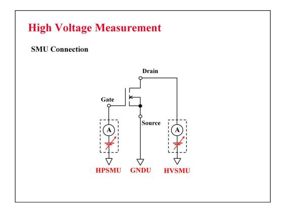
HPSMU can be used for the measurement up to  $200\ V$ . And HVSMU supports the high voltage measurement up to  $3000\ V$ .
