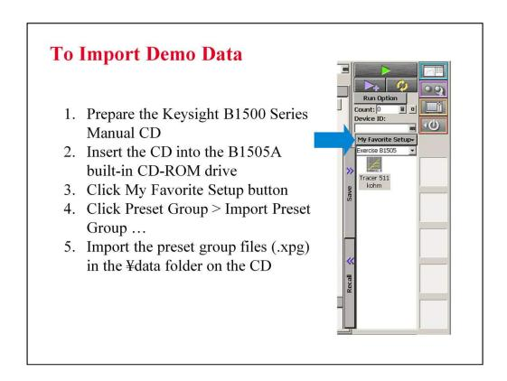
The Keysight B1500 Series Manual CD stores demo data for this class exercise. Insert the CD and import the demo data to the EasyEXPERT database. The Exercise B1505.xpg file contains the test setup data used in this class exercise.
