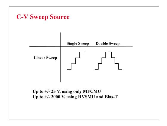
MFCMU supports the linear single sweep and the linear double sweep. The MFCMU can sweep up to a value and then back down (double sweep). This feature is useful when the device must be tested without abruptly removing the forcing condition.
